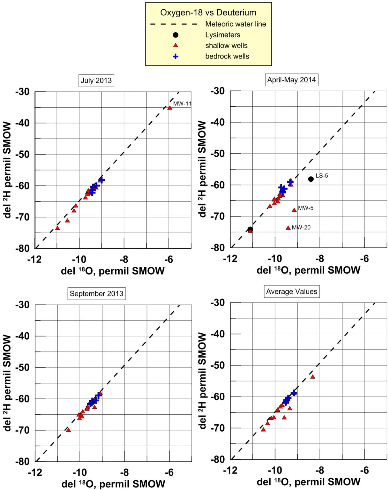
Figure 8. del <sup>18</sup>O versus del deuterium plots for each of the three sampling events and the average of all events. Dashed line shows local meteoric water line from Swanson et al. (2006).
