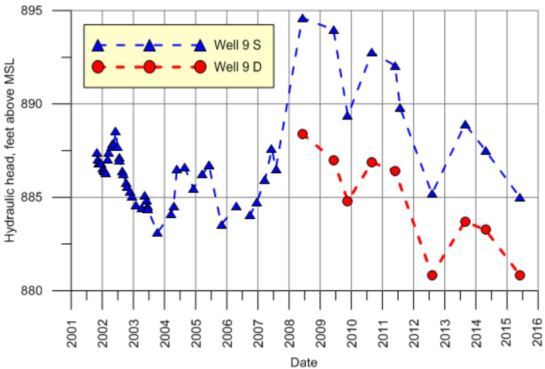
Figure 7. Hydrographs of wells MW9 shallow and MW9 deep
