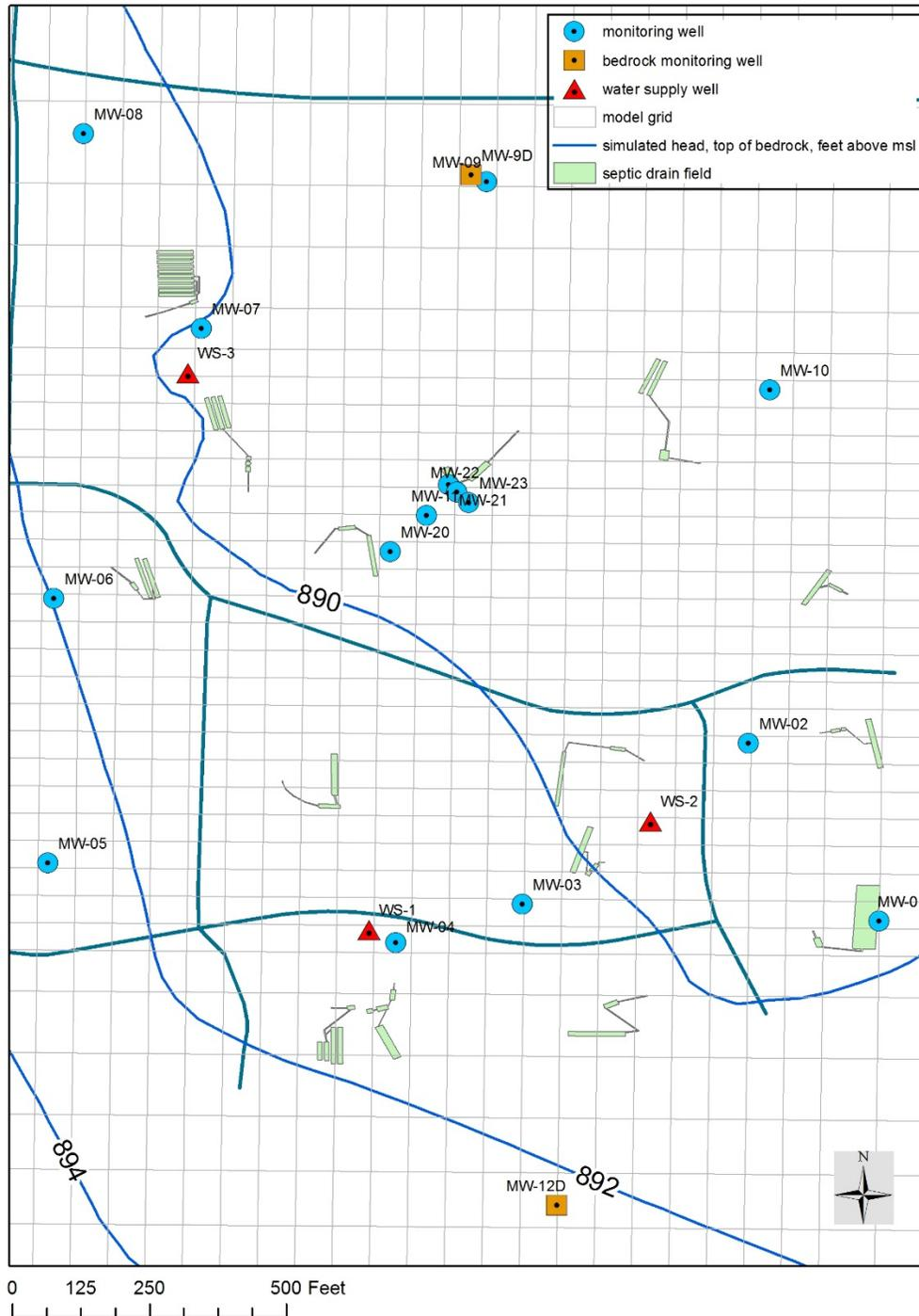
Figure 5. Model grid with simulated water table contours.
