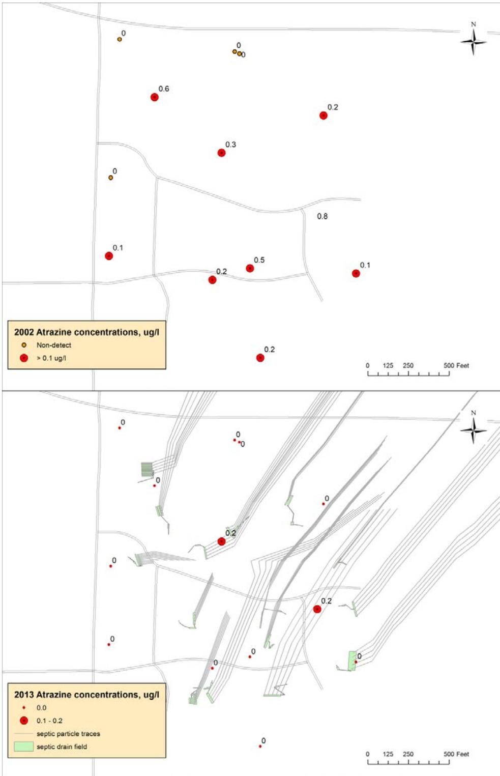
Figure 12. Top: Atrazine concentrations ( $\mu\text{g/l}$ ) in 2002 (prior to development). Bottom: Atrazine concentrations ( $\mu\text{g/l}$ ) in 2013. Gray lines represent forward particle paths from septic drainfields. Light green represents septic systems.
