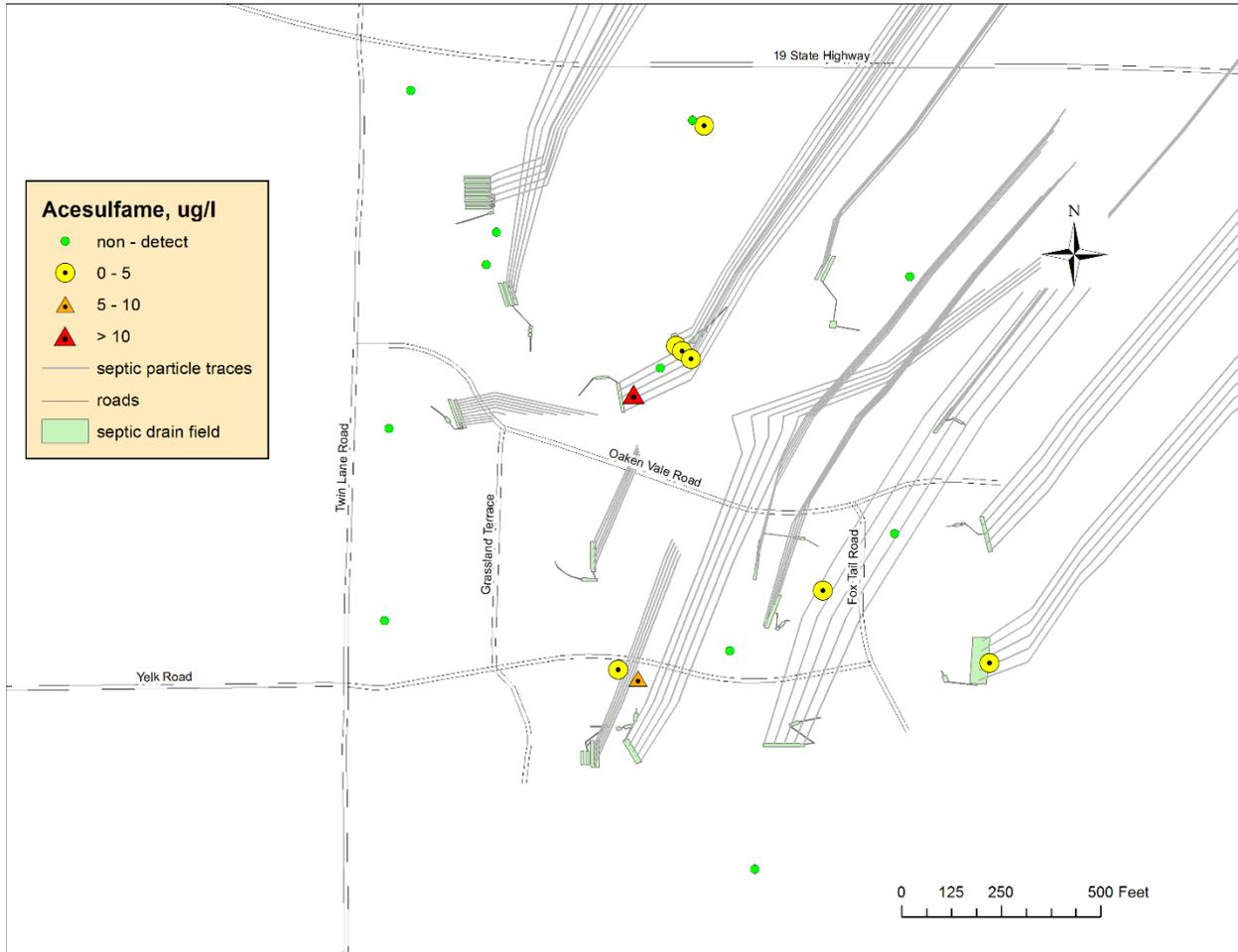
Figure 13. Distribution of artificial sweeteners from 2013 sampling. Gray lines show forward particle tracks from septic drain fields. Septic systems shown in light green.
