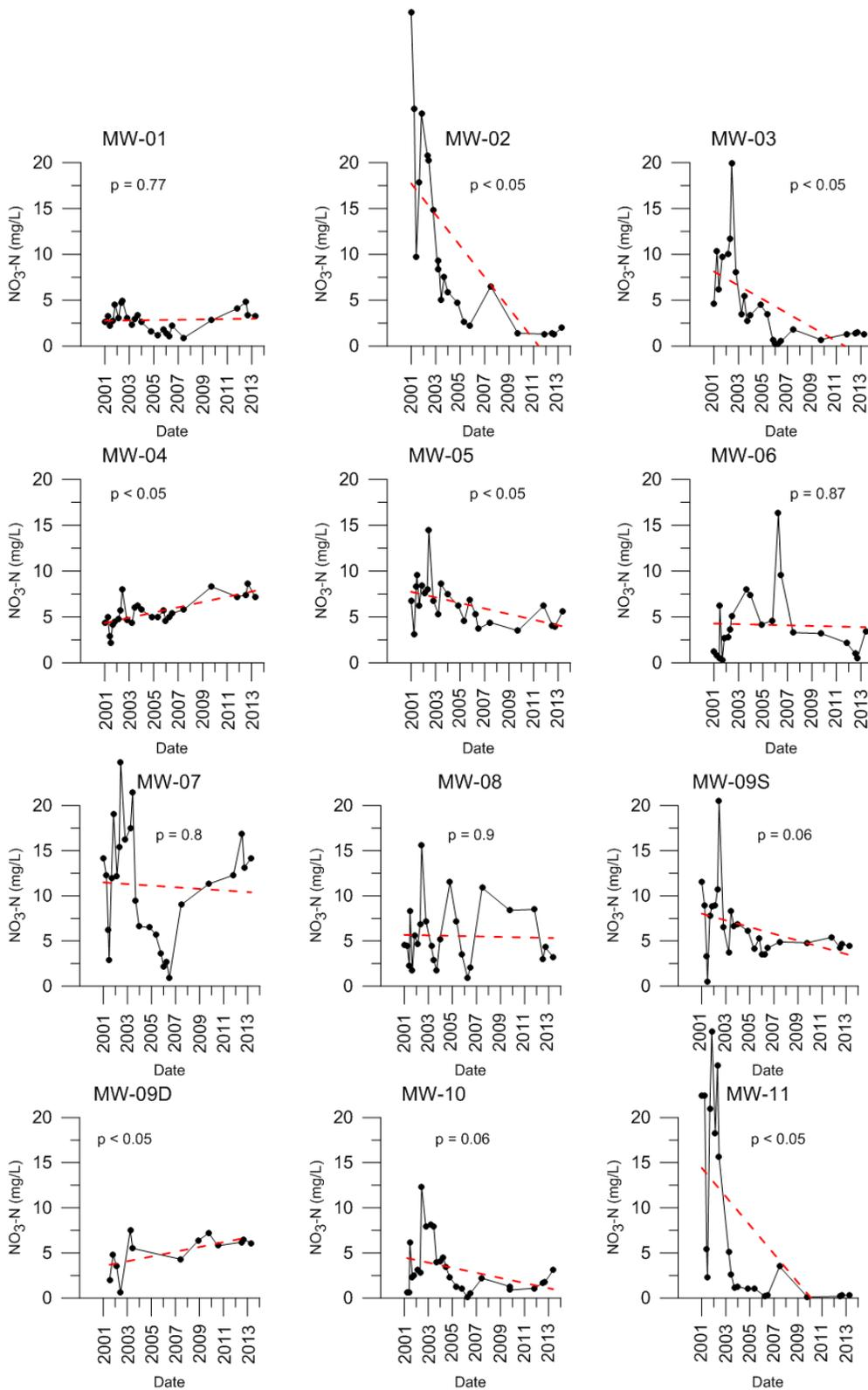
Figure 10. Concentrations of dissolved nitrate (as N) through time at 12 selected wells. Dashed lines indicate linear regression fit, and p-values indicate significance of the regression slope.
