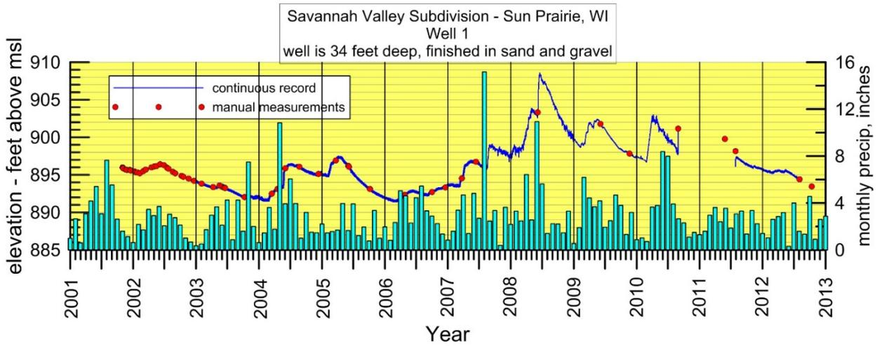
Figure 6. Long-term hydrograph and precipitation record for MW1 in Savannah Valley.
