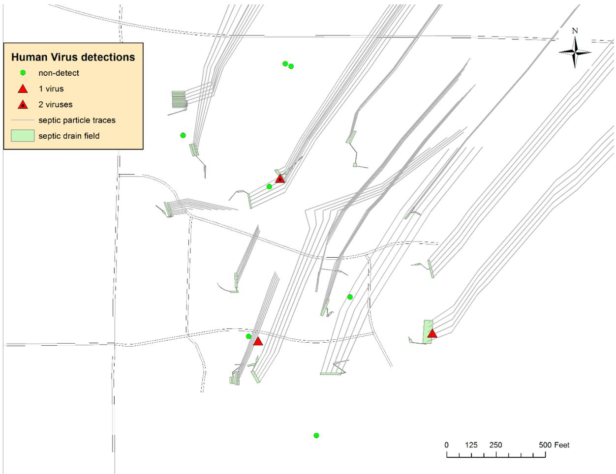
Figure 14. Human virus detections in sampling points in the Savanna Valley study area. Gray lines show forward particle tracks from septic drain fields. Septic systems shown in light green.
