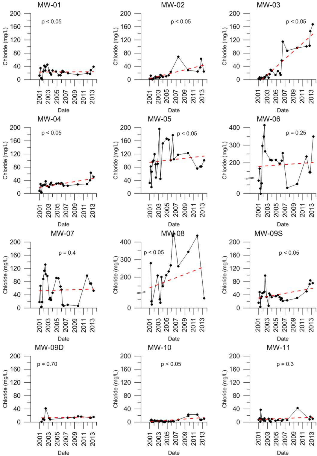
Figure 9. Concentrations of dissolved chloride through time at 12 selected wells. Dashed lines indicate linear regression fit, and p-values indicate significance of the regression slope.
