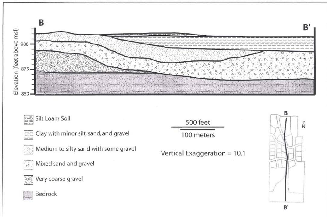
Figure 4. A. East-west schematic cross section through the Savannah Valley Subdivision. B. North-South schematic cross section modified from Wilcox (2003).
