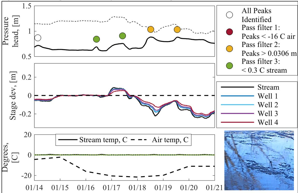
**Figure 9.** Sugar River pressure head, stage deviation, and temperature for 01/14/2016 - 01/21/2016
