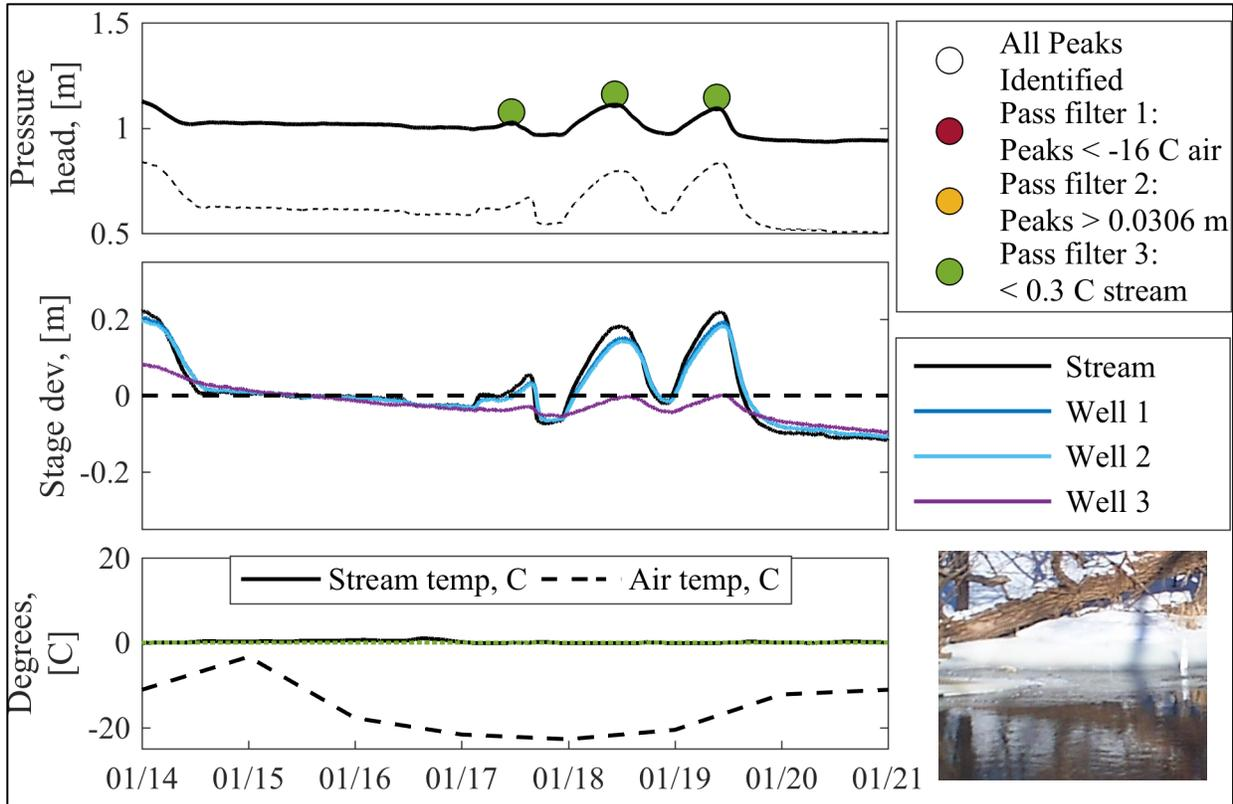
**Figure 8.** Fox River pressure head, stage deviation, and temperature for 01/14/2016 - 01/21/2016
