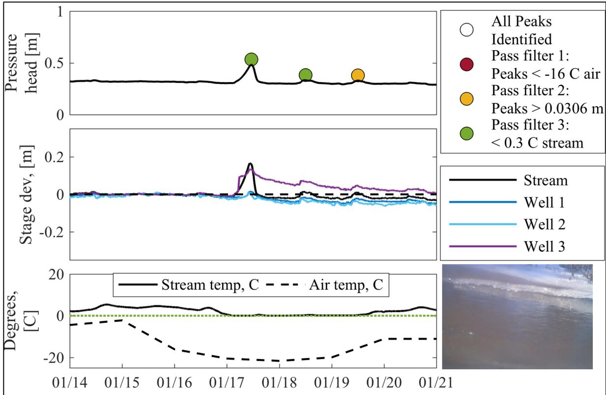
Figure 6. EBP pressure head, stage deviation, and temperature for 01/14/2016 - 01/21/2016
