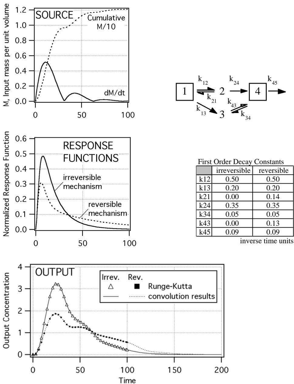
Figure 2-1 Example response function method simulation to model irreversible and reversible linear systems.
