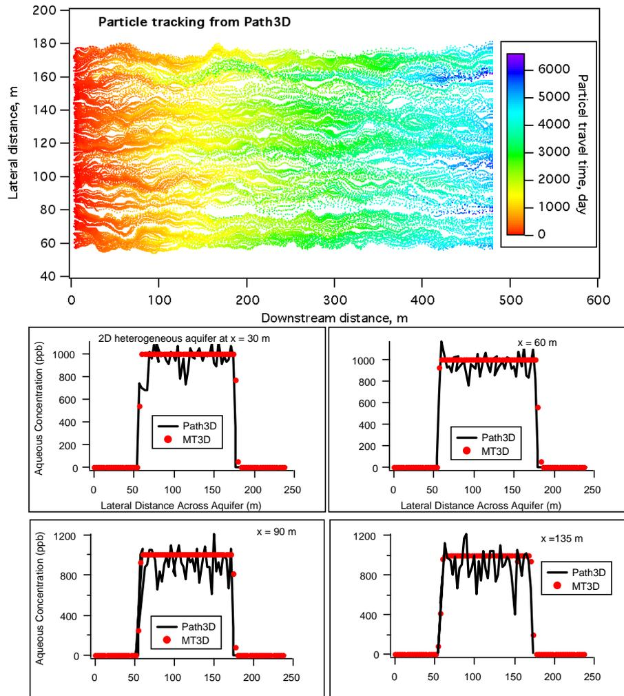
Figure 4-5 Compared with MT3D in the heterogeneous aquifer.
