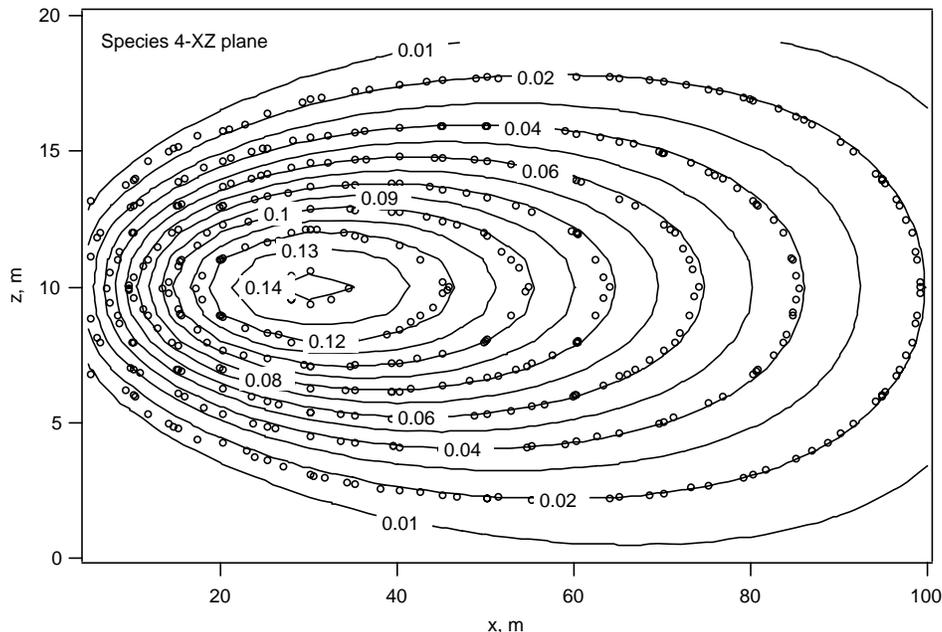
Figure 4-2 Plume simulation at  $t = 500$  d for 4<sup>th</sup> species in a decay chain resulting from rectangular, continuous source of the 1<sup>st</sup> species.
