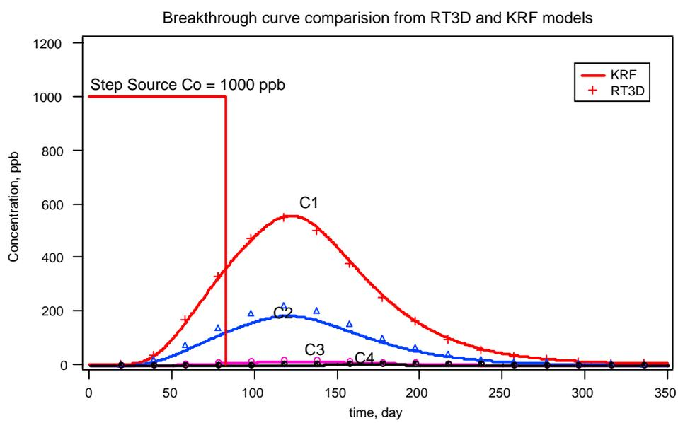
Figure 4-9a Comparison of the four species concentration with KRF approach and RT3D at monitoring point (row 41, column 20)
