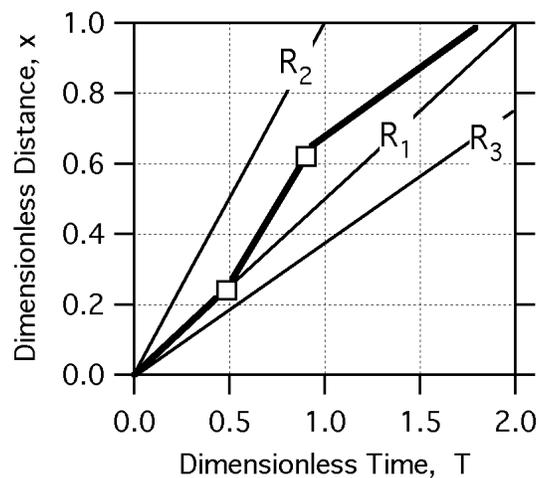
Figure 3-7 Effective trajectory of a particle that degrades sequentially from species 1 to species 3. (considering plug flow and that each species has a different retardation coefficient  $R$ . Particle trajectory is shown in bold. Lighter lines are for nonreactive particles having same retardation coefficients of species 1, 2 and 3.)
