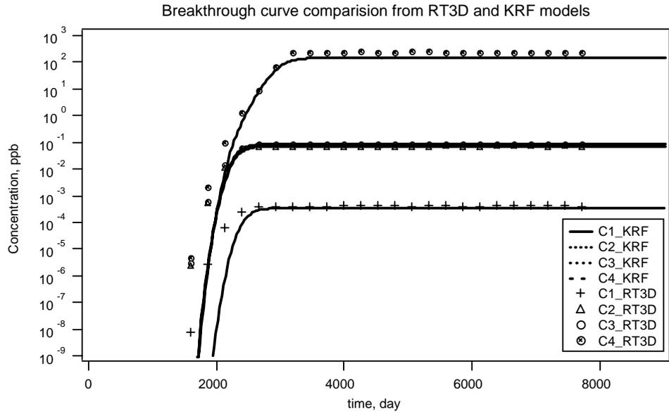
Figure 4-8b Comparison of the four species concentration with KRF approach and RT3D at monitoring point (row 45, column 80)
