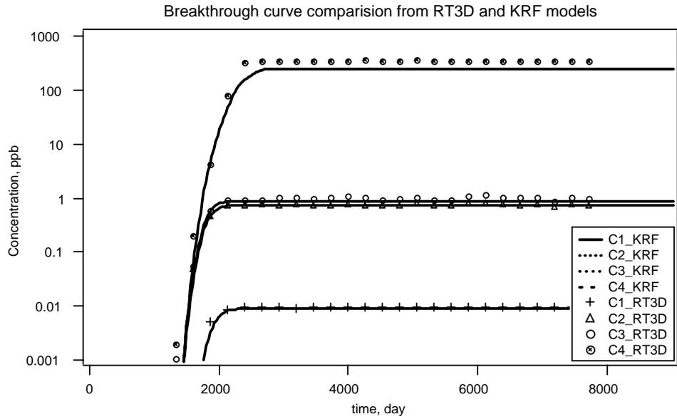
Figure 4-8c Comparison of the four species concentration with KRF approach and RT3D at monitoring point (row 41, column 60)
