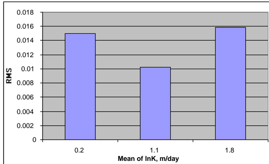
Figure 4-10b RMS of the 4<sup>th</sup> species between KRF model and RT3D model results under different mean of log-normal hydraulic conductivity
