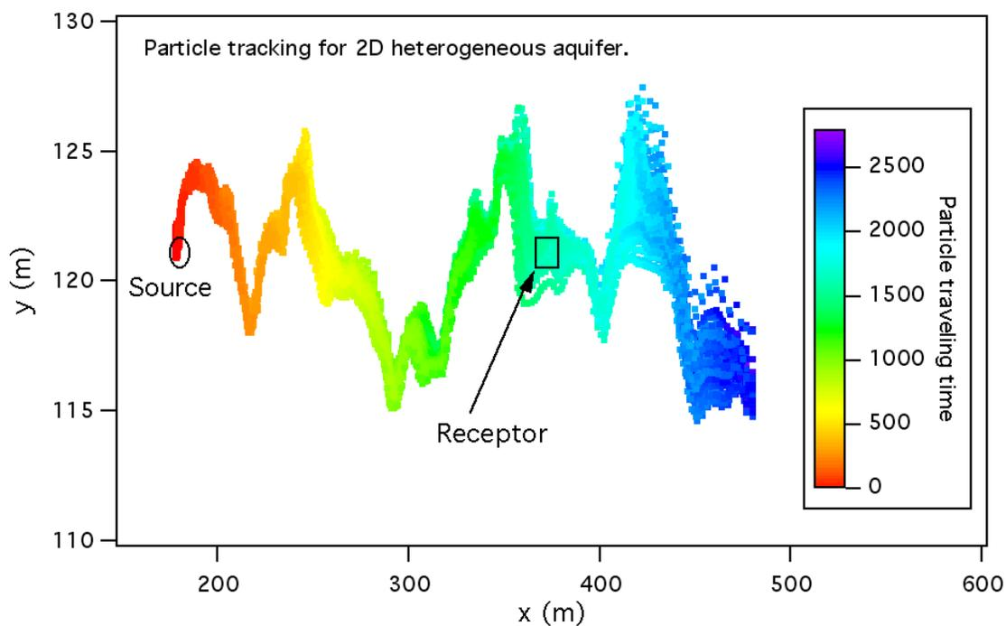
Figure 4-3a Particle tracking path in a 2D heterogeneous aquifer.
