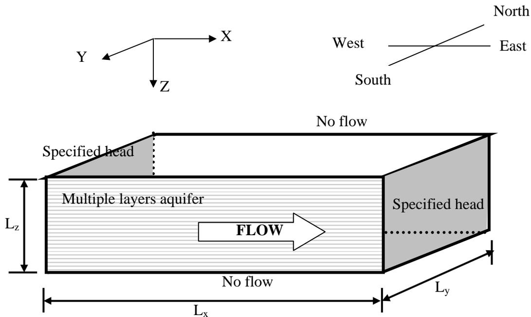
Figure 3-3 Conceptual model of heterogeneous aquifer
