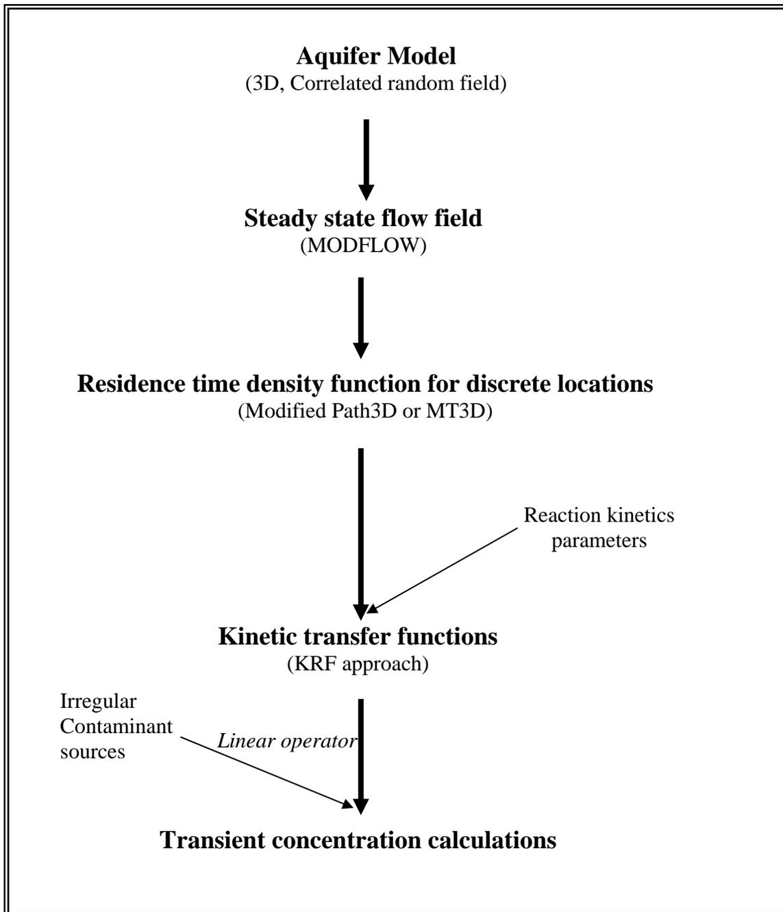
Figure 3-1 Kinetic response function modeling sequence scheme
