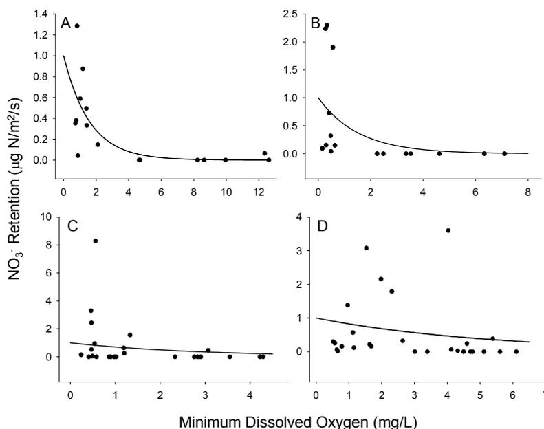
Fig. 3 Nitrate retention plotted against  $DO_{\min}$  at Radley-West (A), Big Roche a Cri (B), Radley-Suhs (C) and Emmons Cr. (D). The general form of the nonlinear model is nitrate retention =  $\exp(-x DO_{\min})$ . The coefficients and  $r^2$  are 0.626, 0.677 (A), 0.653, 0.465 (B), 0.349, 0.21 (C), 0.190, 0.254 (D).
