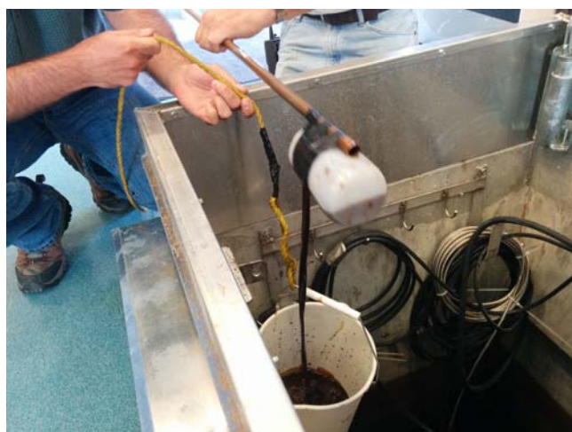
Figure 4. Collection of Mn oxide slurry from Well 29 Mn removal system.
