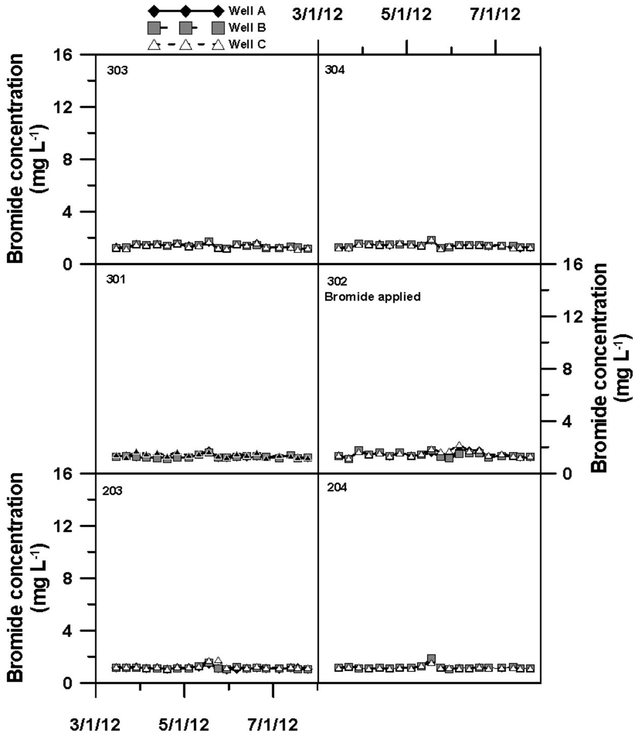
Figure 3. Bromide concentrations in the north six plots of the second field where bromide was applied on 9 March 2012. The first sample date represents the day on which bromide was applied.
