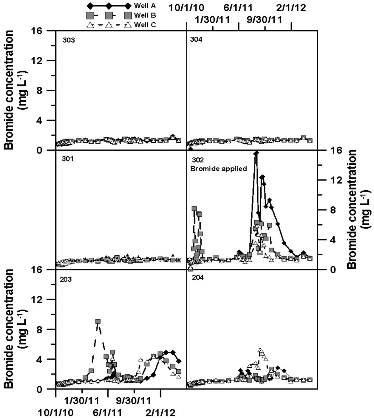
Figure 1. Bromide concentrations in the north six plots of the first field where bromide was applied on 14 October 2010. The first sample date represents the day on which bromide was applied.
