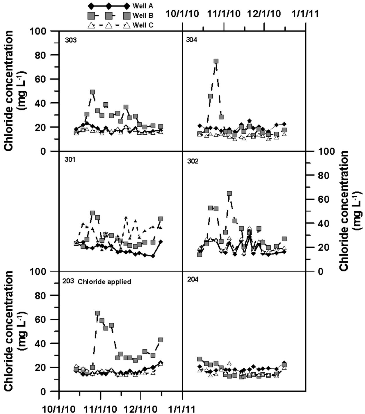
Figure 5. Chloride concentrations in the north six plots of the first field where chloride was applied on 14 October 2010. The first sample date represents the day on which chloride was applied.
