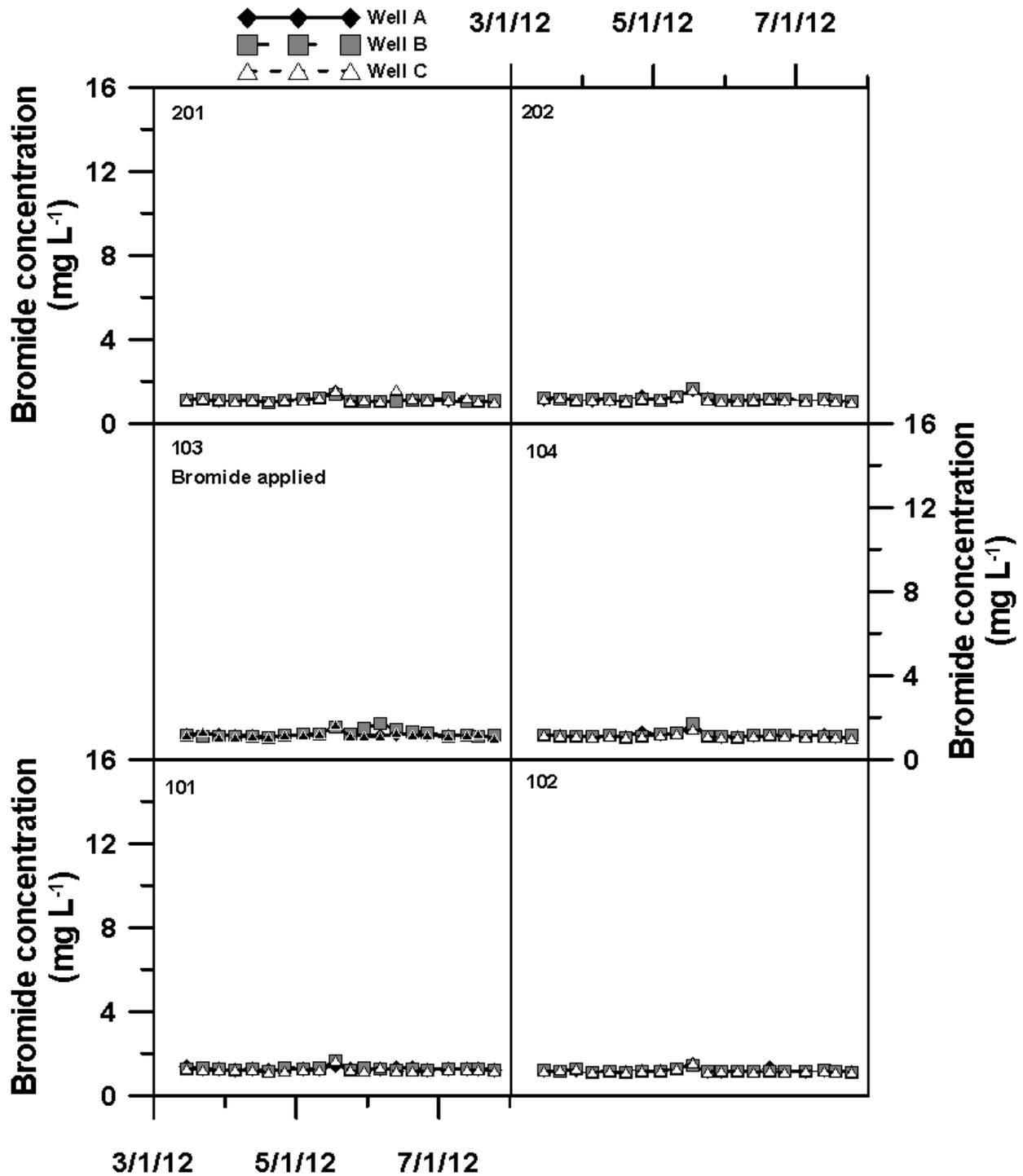
Figure 4. Bromide concentrations in the south six plots of the second field where bromide was applied on 9 March 2012. The first sample date represents the day on which bromide was applied.
