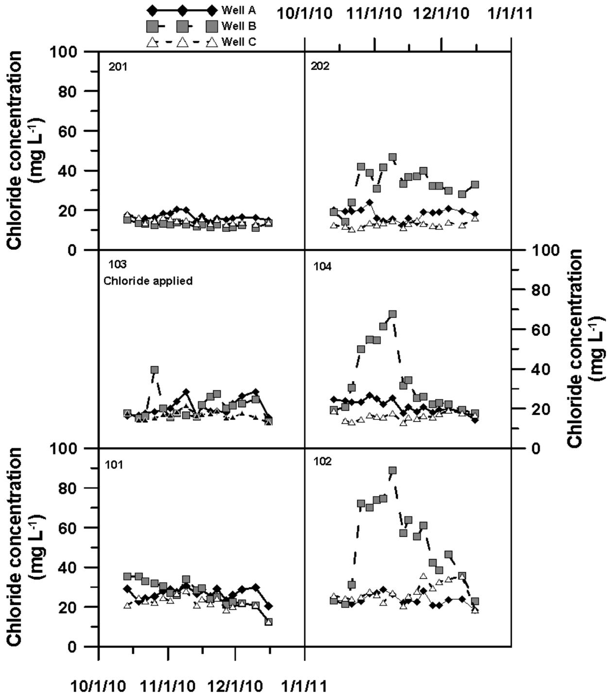
Figure 6. Chloride concentrations in the south six plots of the first field where chloride was applied on 14 October 2010. The first sample date represents the day on which chloride was applied.
