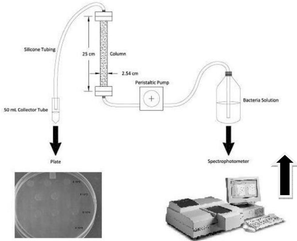
Figure 2.1 Schematic of the Flow System
