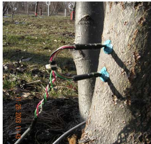
Figure 2. Diagram of thermal dissipation probe (Dynamax, Inc) and insertion into hybrid poplar.
