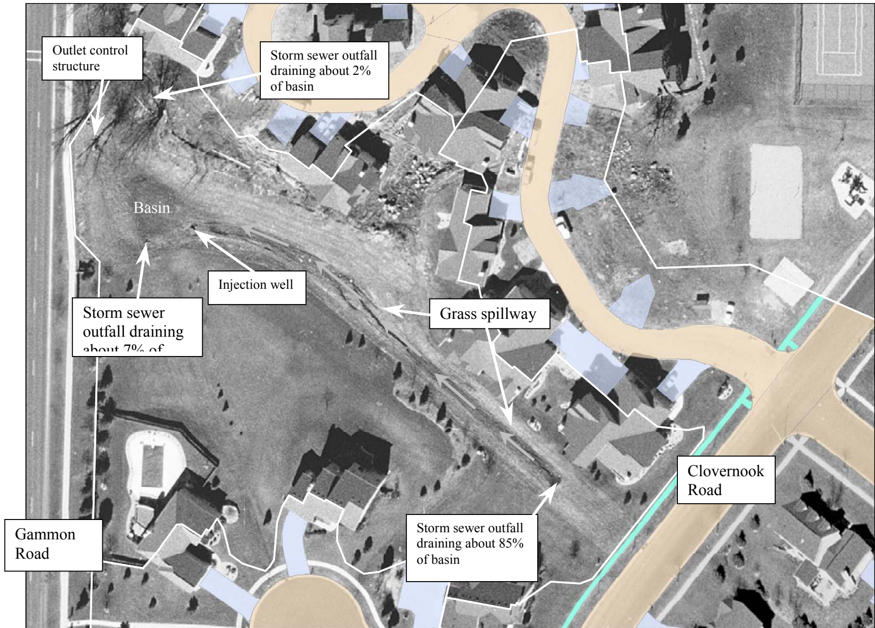
Figure 3. Aerial view of Stonefield Infiltration Site showing location of sewer outfalls, the outlet structure and the injection well
