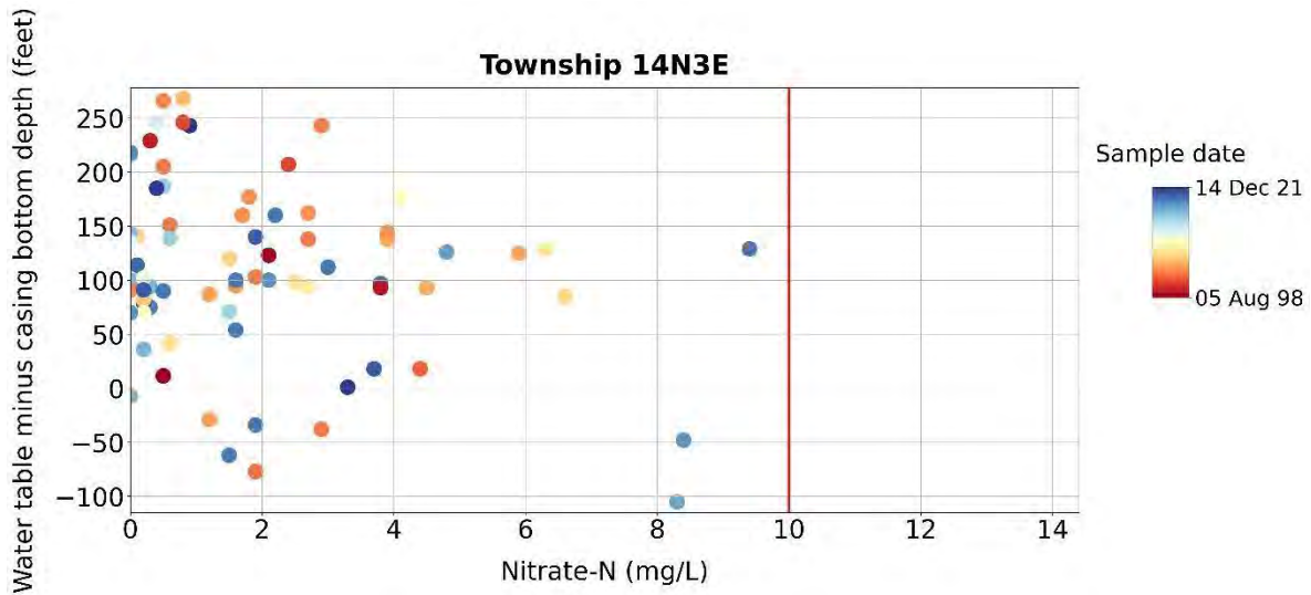
Figure C 2. Township 14N3E. (top) Yearly average nitrate concentration versus year of sampling. Dashed line indicated linear regression of the data. R^2 is the goodness of fit of the linear relationship. (bottom) Nitrate concentration versus the difference between the static water table and the casing depth. Color refers to the sampling date: the oldest measurements are marked with a red color, the most recent measurements are marked with a blue color.
