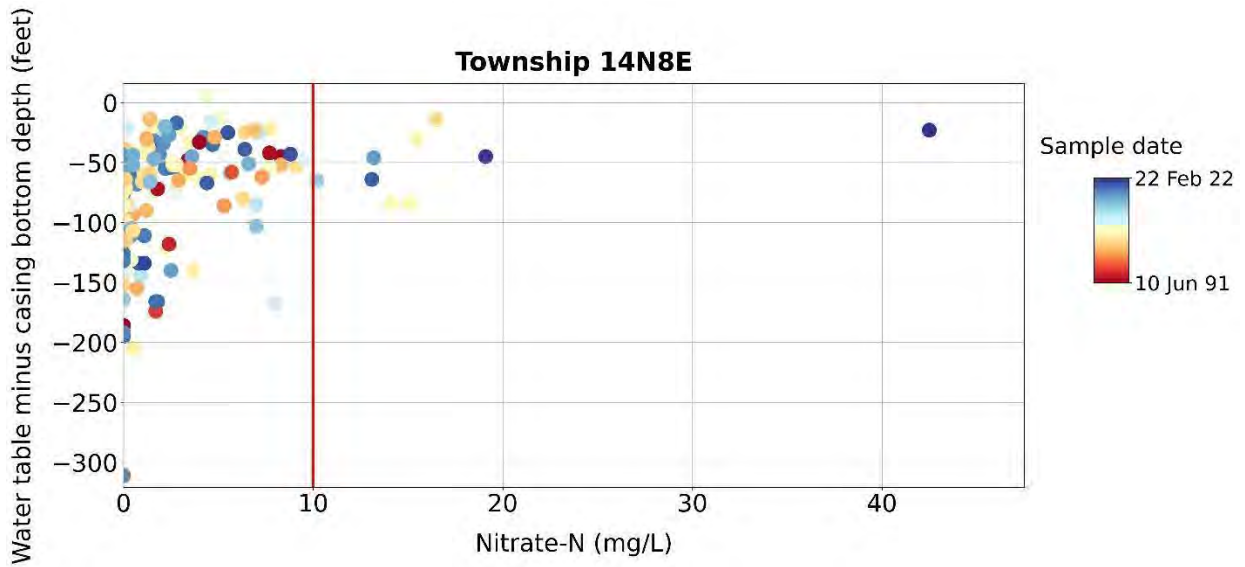
Figure C 7. Township 14N8E. (top) Yearly average nitrate concentration versus year of sampling. Dashed line indicated linear regression of the data. R^2 is the goodness of fit of the linear relationship. (bottom) Nitrate concentration versus the difference between the static water table and the casing depth. Color refers to the sampling date: the oldest measurements are marked with a red color, the most recent measurements are marked with a blue color.
