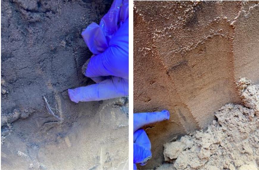
*Figure A.37: Fingering shown at multiple depths (>55 cm) after excavating the short-term infiltration area.*
